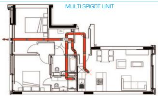
$\textbf{TYPICAL MICROBOX SAVING-£249 PER SYSTEM-less ducting, fewer fire dampers and less coring, easier to install a substitution of the property of the propert$
